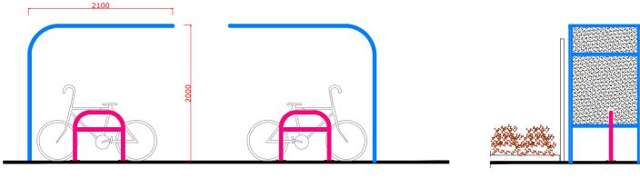
CYCLE AREA CYCLE AREA SECTION B-B SECTION A-A SCALE: 1/50 SCALE: 1/50
